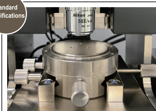
Sample holder * Sample size: 50 mm diameter \times 3.5 mm thick
