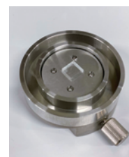
Underwater sample holder * Sample size \phi 20\text{mm} \times 3\text{mm} * Schematic Sample Indenter solution
